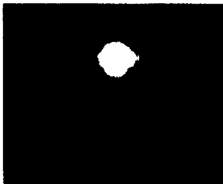
Fig. 8. The picture of the extracted beam on the monitor screen.
