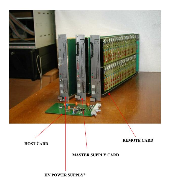
\* HV Power Supply is the module for small size system especially. The total current is  $2.5\ \text{mA}$ .
