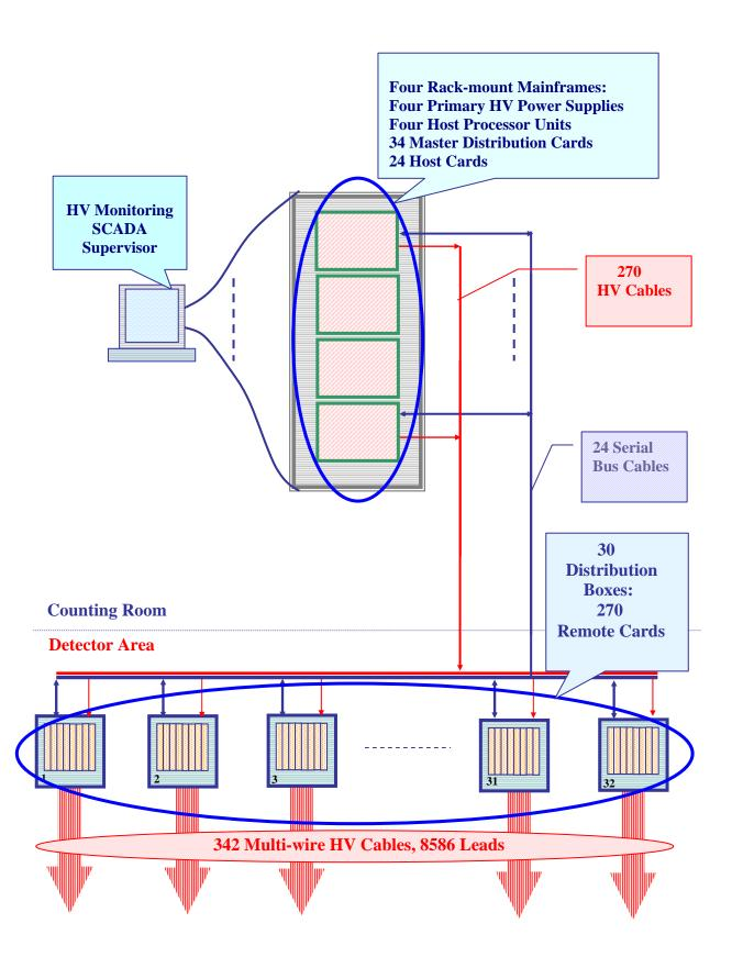
Fig.4. HVM System Approaching (8208 Channels)
