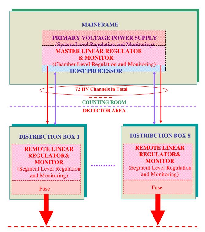
Up to 2592 HV Channels in Total (4 Mainframes per 8856 Channel EMU CMS System)
