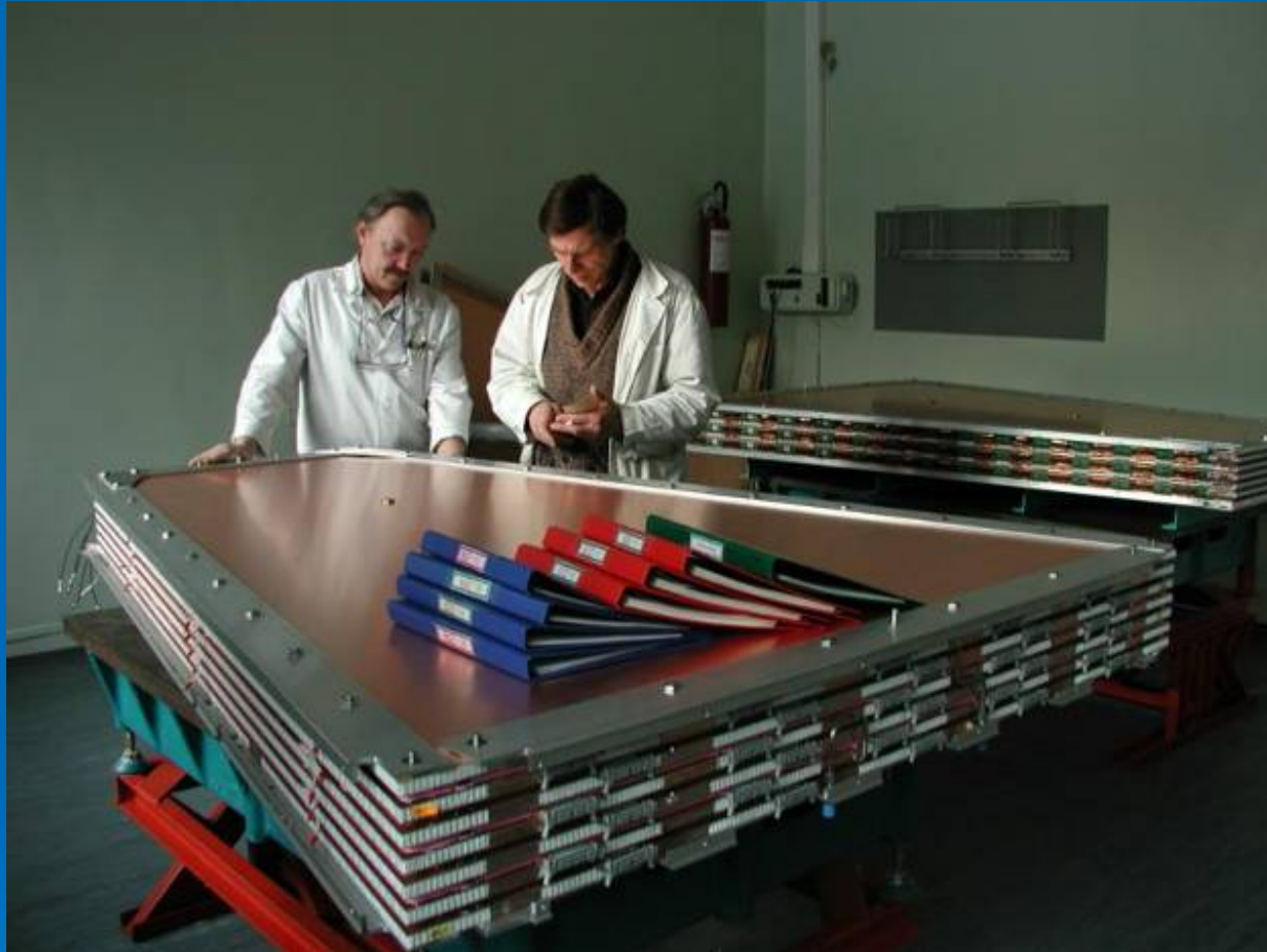
Assembled CSC ready for final tests
