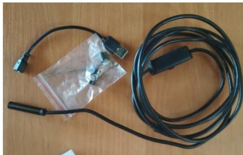
7 mm waterproof Endoscope. 720p
