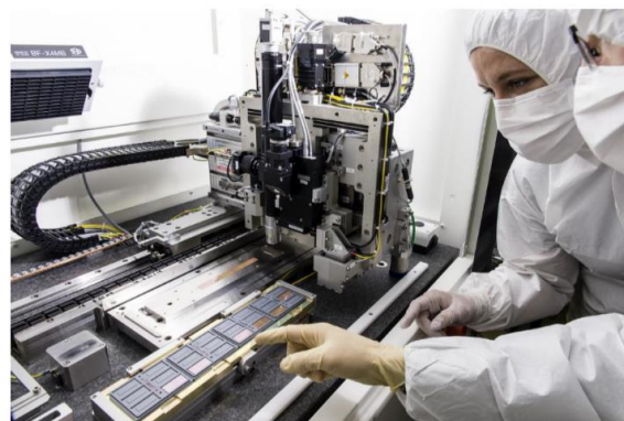
Chip alignment/gluing with ALICIA7 machine
