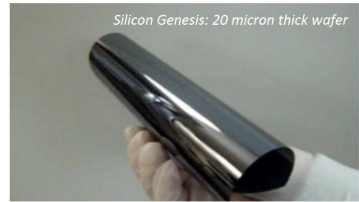
Ultra-thin chip (<50 \mu\text{m} ): flexible with good stability
