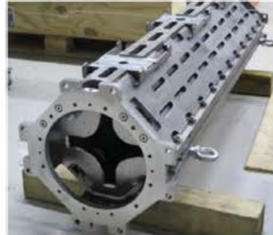
First SIS100 s.c quadrupole yoke and s.c. coil at JINR (Russia/Germany)
