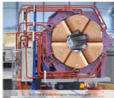
FOS (first of series) sextupole magnet delivered. SAT successful, Series released (Denmark).
