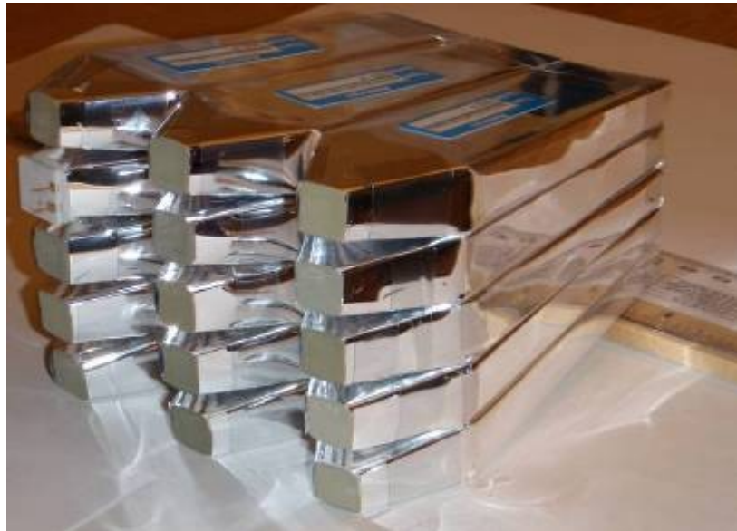
R3B Calorimeter Demonstrator: 15 CsI(Tl) elements
