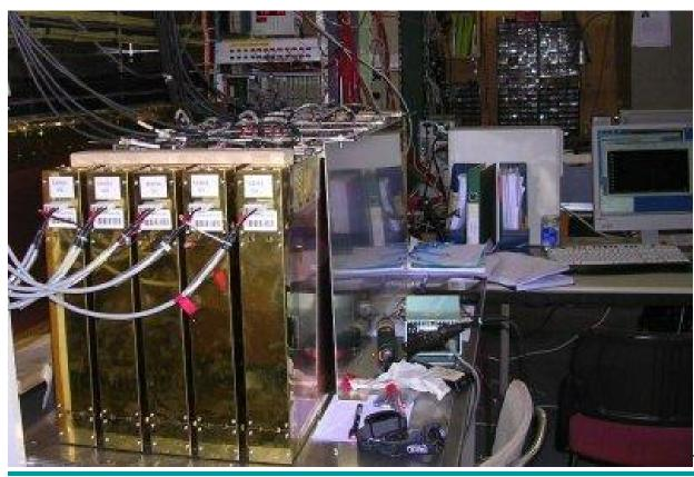
5 chambers can be tested simultaneously
