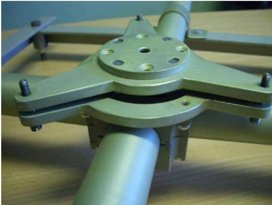
Hexagon mirror tuning mechanism
