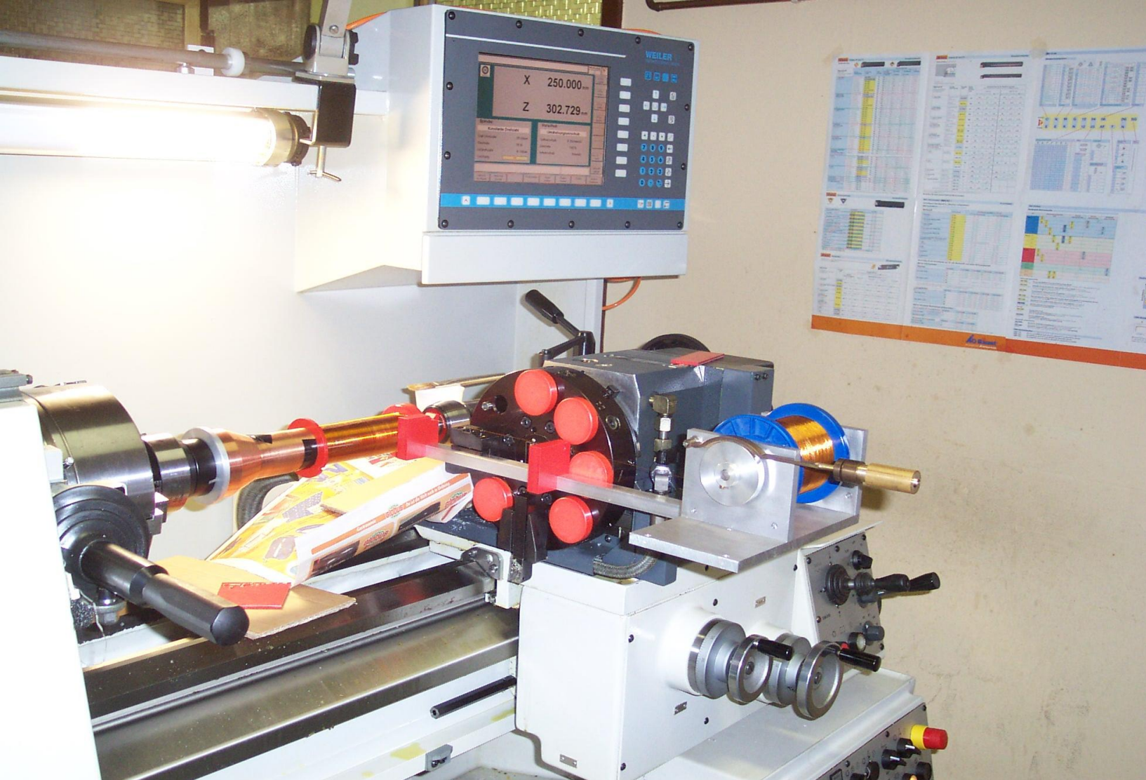
Coil winding in Mainz workshop Glueing with Epoxy
