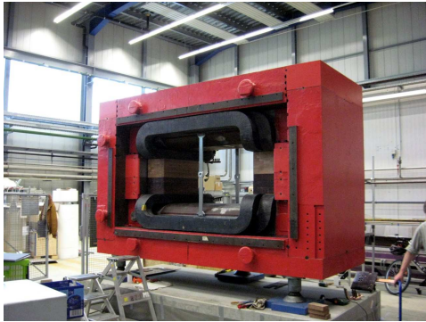
Figure 3: Photo of the magnet after gap extension and ready for the field measurement at the GSI.
