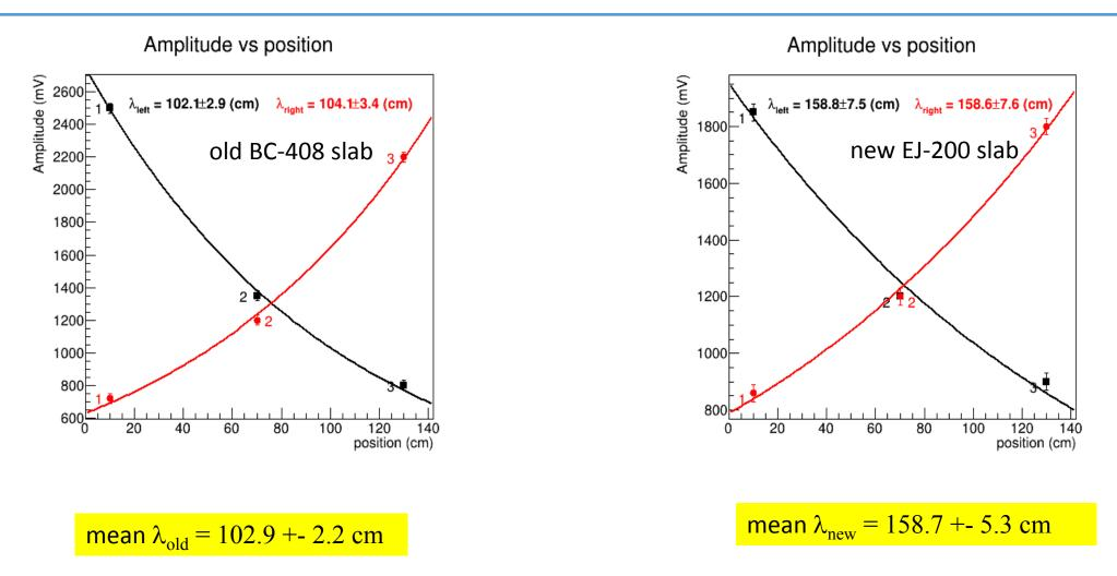
The measured attenuation length for new slab is about 1.5 times longer. That is in coincidence with scintillator material datasheets.
