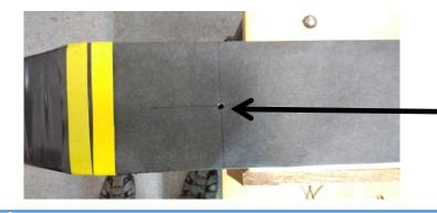
Three 5mm diameter holes in the wrapping materials were made along the slab. One in the center and one at a distance of 10 cm from each side.
