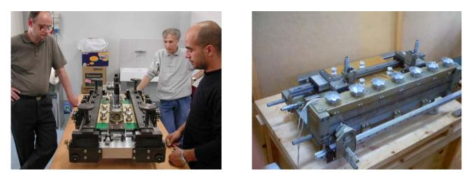
Fig. 2. The PCB trimmers developed for preparation of the slats for stations 3, 4, 5 (left) and for station 2 (right) at PNPI
