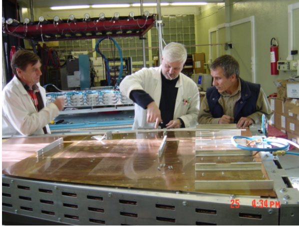
Fig 5. Installation of the on-chamber electronics
