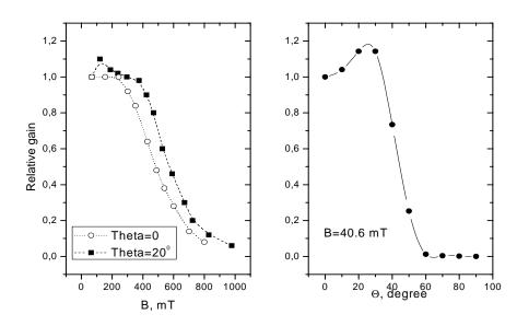
Fig. 8. Magnetic properties of fine-mesh FEU-187
