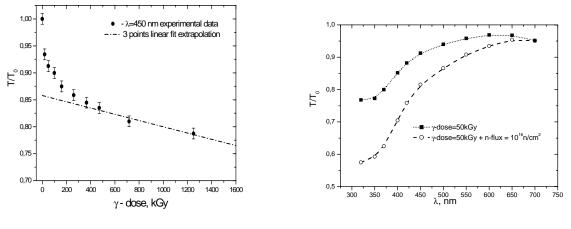
**Fig. 3.** The linear extrapolation of  $T/T_0$  data at the different doses of <sup>60</sup>Co  $\gamma$ -irradiation
