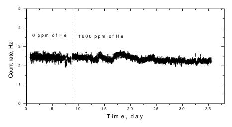
Fig. 7. Dark noise count rate in N<sub>2</sub> atmosphere with 1600 ppm of He admixture
