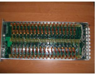
Fig. 2. 36-channel Remote Distributor
