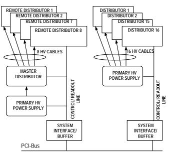
Fig. 1. Block diagram of the HVDM system
