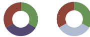
Fig. 2. Illustration of Scatter-Pie when derive three dimensions. Each Scatter-Pie is divided into three parts to indicate user knowledge over these three dimensions. Special colors (red, green, blue) are filled when user knows this data object over this dimension, and gray is filled when user does not know this data object over this dimension. (Color figure online)
